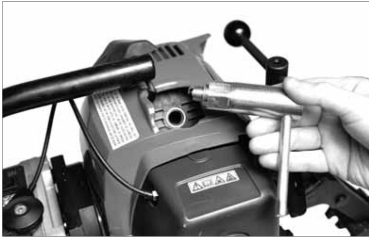
FIG. 29 – SPARK PLUG CLEANING
