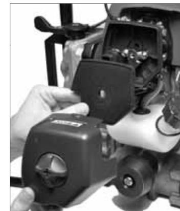
FIG. 27 – FUEL FILTER CLEANING
