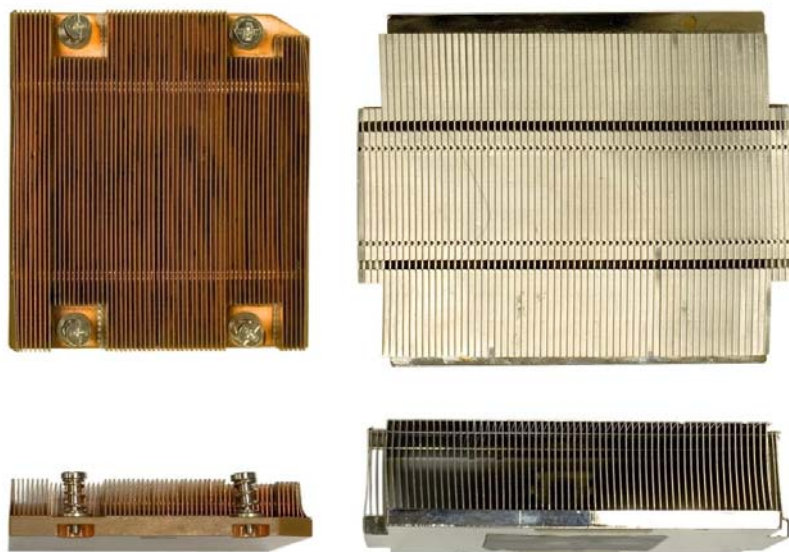
Figure 9. Processor heat sink using fully ducted design (left) versus traditional heat sink in a 1U rack-mount server (right)
