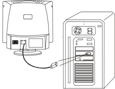
☞ *To connect the monitor to an older type Apple Macintosh through a D-Sub cable, you need to use an Apple Macintosh signal adaptor to connect the video signal port of your computer to the monitor signal cable. Adaptors are available from Mitsubishi Electric Australia. Please contact your computer dealer for more information.*
