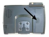
The main switch is on the left side of the battery.
