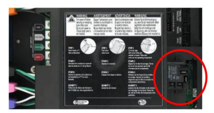
4) Move the heater management jumper to the right position (disabled). Jumper 7 for North American boards and jumper 8 for Export boards.
