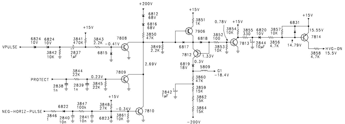
FIGURE 14 - SWEEP FAILURE DETECTION AND BLANKING
