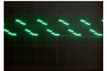
Pb from HD-DW module measured on Pin 3 of 1411.
