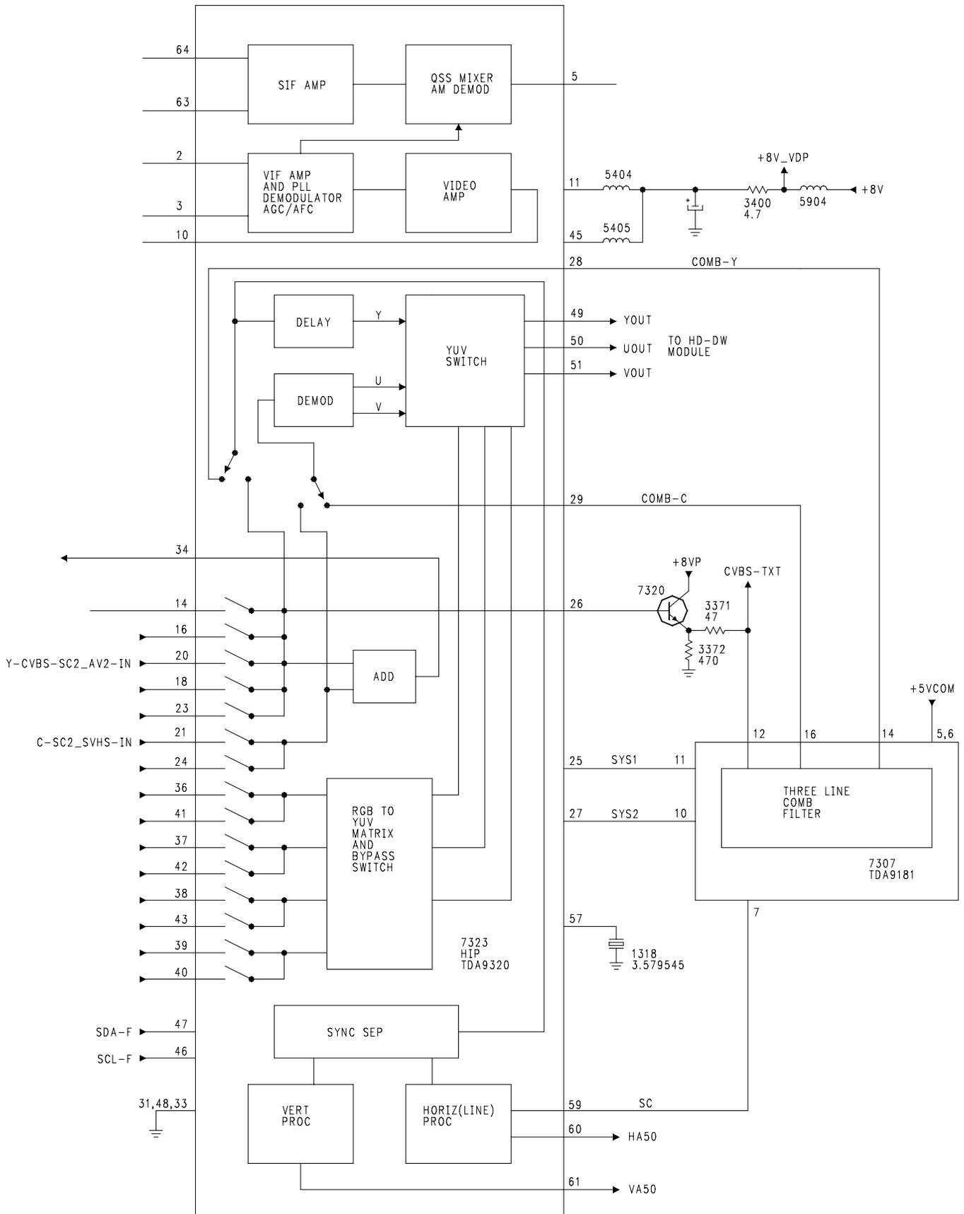
FIGURE 18 - NTSC SSB SIGNAL PROCESSING
