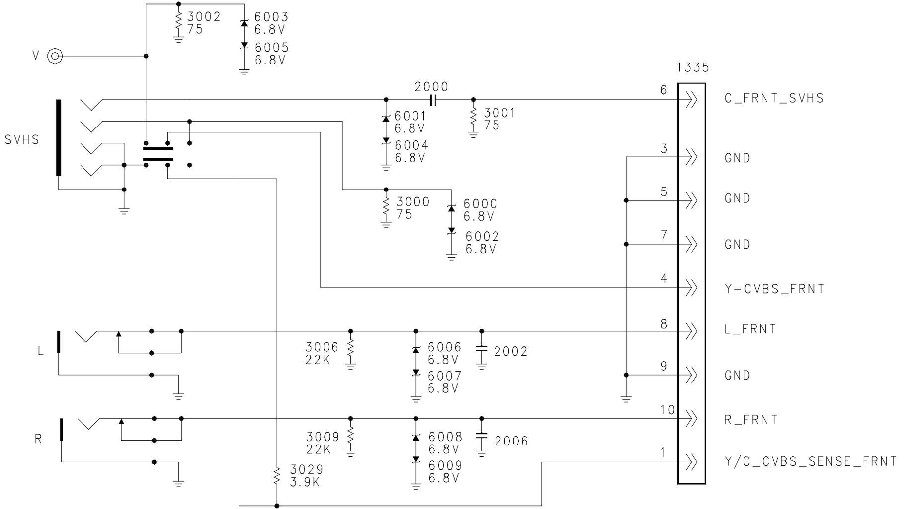
FIGURE 17 - SSM NTSC AV INPUTS AND SWITCHING
