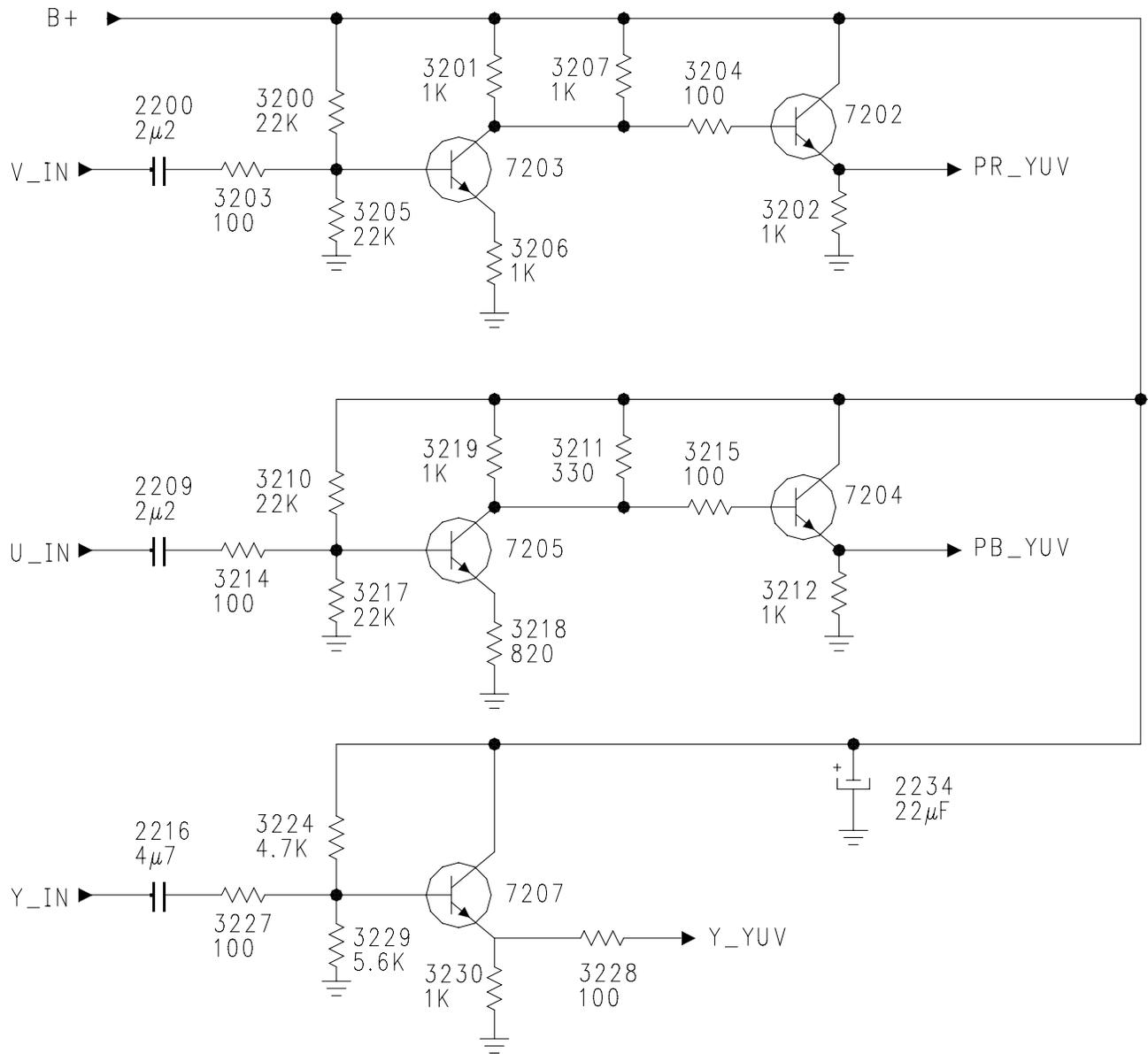
FIGURE 22 - YUV TO Y Pb Pr CONVERTER
