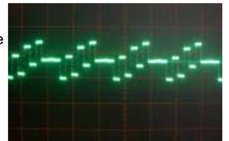
Pr from HD-DW module measured on Pin 5 of 1411.
