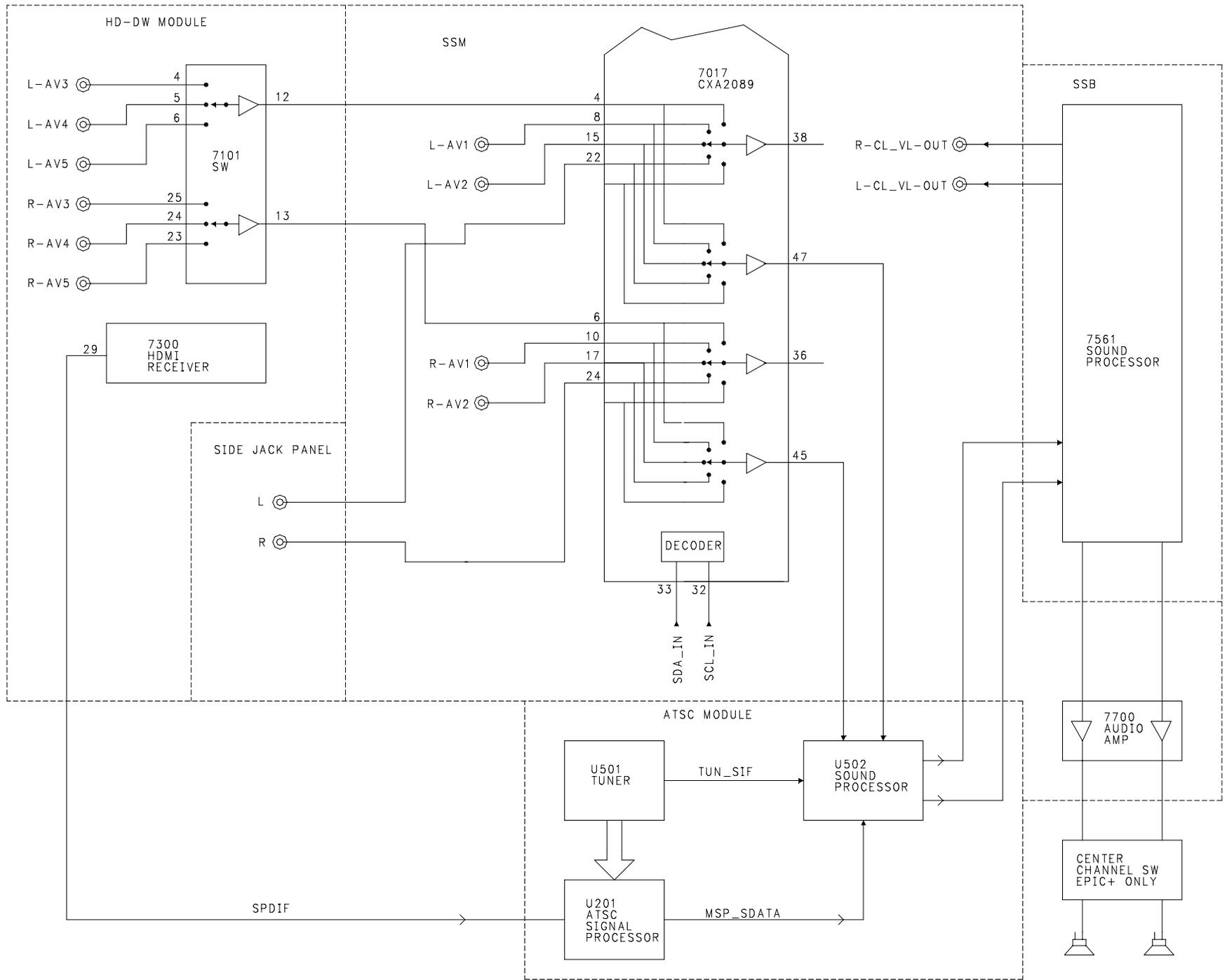
FIGURE 32 - SSB AUDIO PROCESSING
