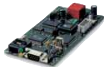
The UPS comes with an expansion slot for optional communication boards such as Netman and MultiCom.
