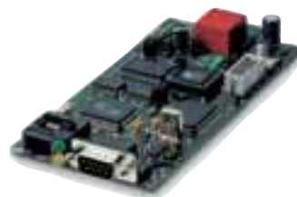
The UPS comes with an expansion slot for optional communication boards such as Netman and MultiCom.
