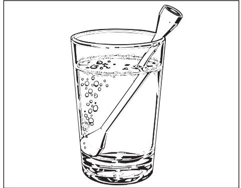
When heating liquids, milk, sauces etc., using microwave heat without the boiling rod, the boiling point of the liquid may be reached without the production of typical bubbles. The liquid does not boil evenly throughout. This so-called 'boiling delay' can cause a sudden build up of bubbles, when the container is removed from the oven or shaken. This can lead to the liquid boiling over suddenly and explosively. Danger of burning.
