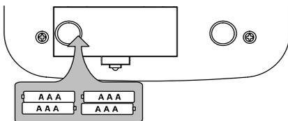
Change the batteries when the
