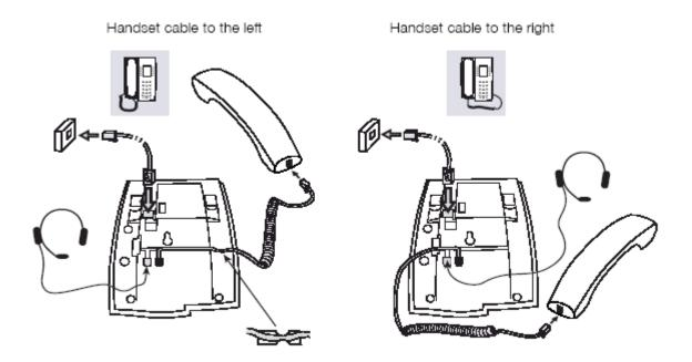
You can put the cable to the handset notch underneath the telephone. The cable to the exchange has to be plugged in "LINE" and the handset cable has to be plugged in "HANDSET".
