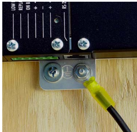
Figure 21. Securing the Ground Wire Lug
