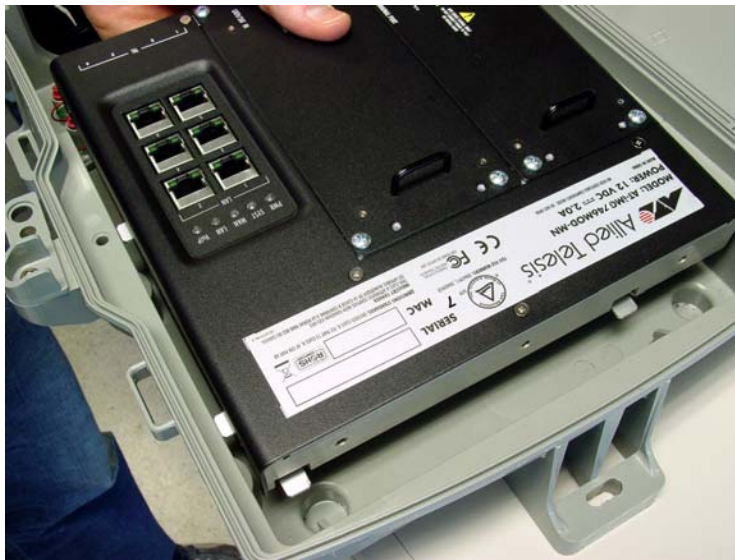
Figure 5. Sliding the gateway into the Enclosure (Tabs into the Notches)
