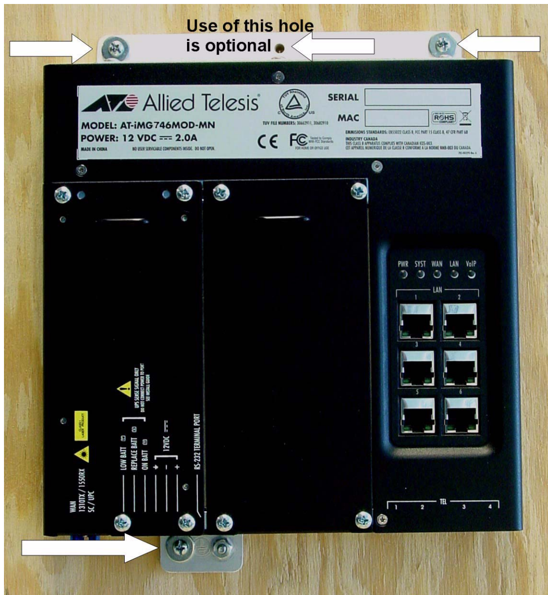
Figure 20. Securing the Gateway to the Mounting Surface
