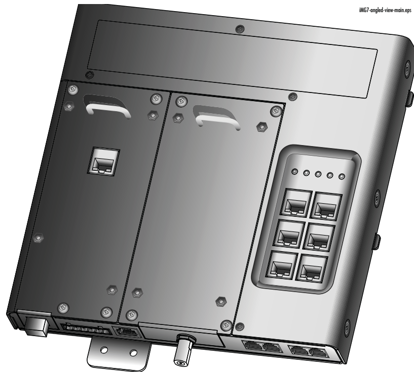
Figure 3. The AT-iMG746MOD Electronics Unit (with Gig BiDi WAN Module with Gig LAN RJ-45 Port)
