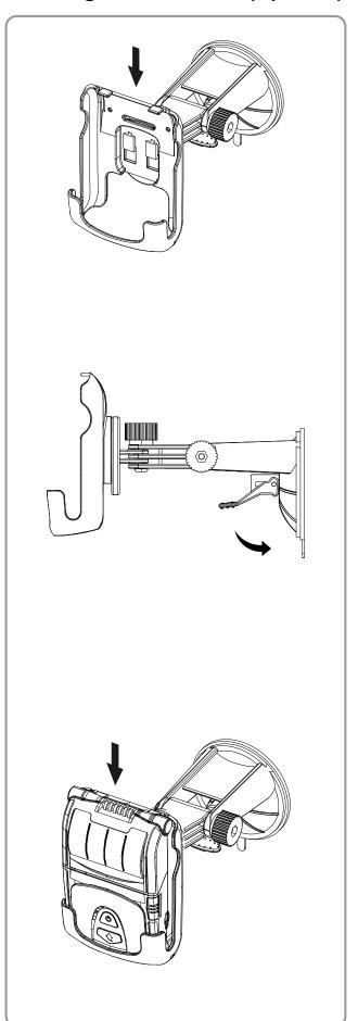
1) Assemble the vehicle holder to the mount.
