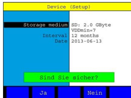
Press **F2** to format the storage medium, or **F4** to abort the formatting; during the formatting, all data contained on the medium (e.g. measured values) will be deleted irretrievably.
