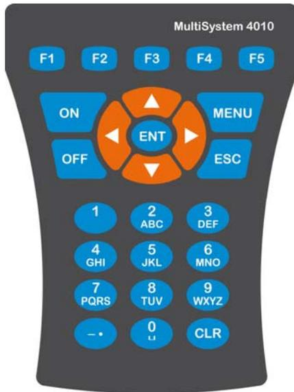
The MultiSystem 4010 is equipped with a valuable keypad that is insensitive against humidity and dirt. The 26 keys are occupied as follows:
