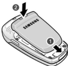
5. Make sure that the battery is properly installed before switching on the phone.
