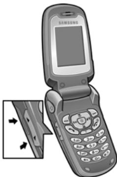
In Idle mode, you can also adjust the ring volume using these keys while the phone is open.
