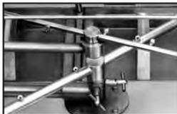
Unique pull-pin design allows wash arms to be easily removed for cleaning.
