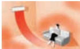
During heating the near-vertical flaps direct air to the floor to quickly warm the room.
