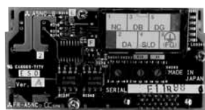
FR-V500 series plug-in option example : FR-A5NC
