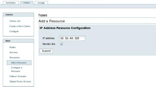
Enter the IP address reserved for the service and select the *Monitor Link* check box. Click *Submit* to create the IP address resource. The IP service resource should now be listed using the /sbinip addr list command. Note that interface eth3 (the public NIC) lists both the external system IP address as well as the IP resource address (10.16.40.165).
