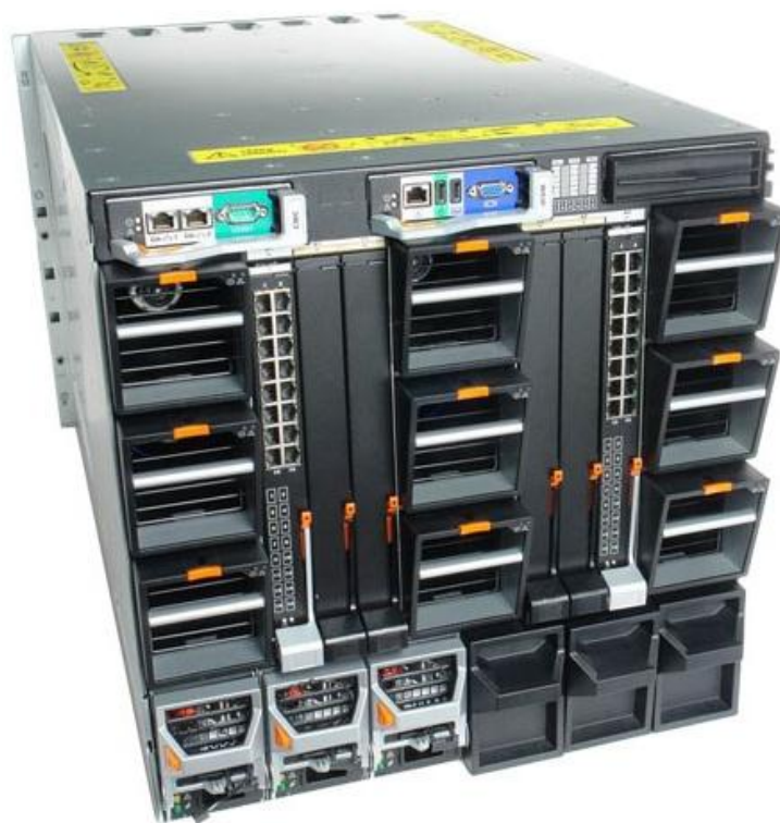
Figure 11. Installed CMC, I/O Module, and Power Supply Blanks
