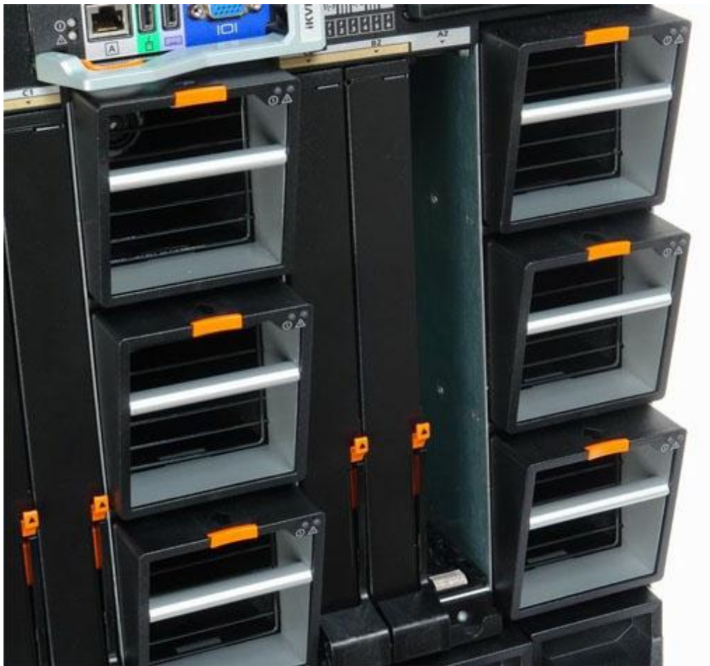
Figure 10. I/O Module and One Open Slot Needing to be Filled
