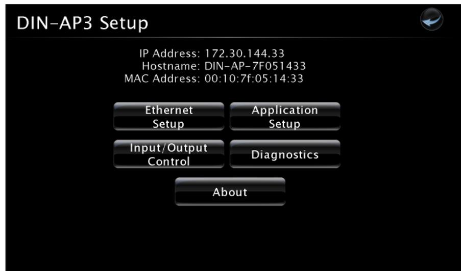
The “DIN-AP3 Setup” menu displays the IP address, hostname and MAC address of the device. It also allows access to various setup and programming screens. The “DIN-AP3 Setup” menu contains buttons for **Ethernet Setup**, **Application Setup**, **Input/Output Control**, **Diagnostics**, and **About**, as shown in the illustration above.
