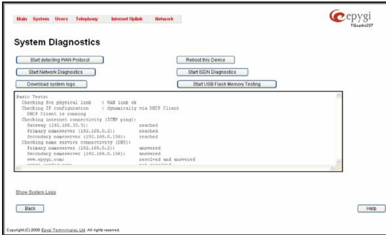
Fig. I-52: System Diagnostics - Network Diagnostics page
