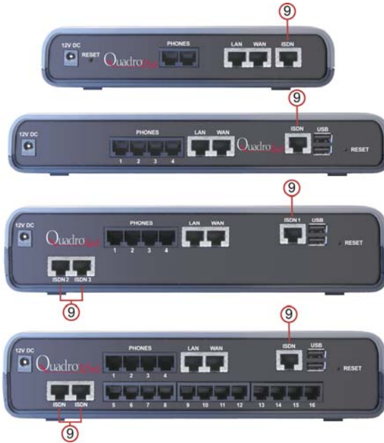
Fig. I-3: ISDN/Ethernet flavored Quadro's Connectors Panels in plastic enclosure
