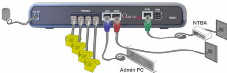
Fig. I-12: Installation: Quadro4xi used as an Internet Access Router
