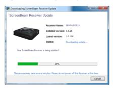
**5.** The firmware is transferred to the Display Adapter. Do not power off the Display Adapter during this transfer.
