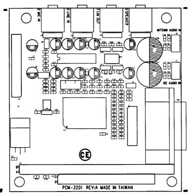
§ Pin No.1,2,5,4,5 OF CN2, CN3, CN4 and CN5 are 1.2x0.6mm availables. § FIRST LAYER IS COMPONENT SIDE.
