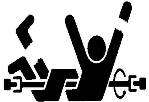
**Operating without guards could result in serious injury or death. Machinery in operation can grab, crush, cut, mangle and dismember. Do not operate without adequate guards in place.**
