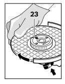
Lock the grinder spindle with the spindle lock button **1**. To tighten the quick-clamping nut, firmly turn the grinding disc in clockwise direction.
