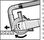
Switch on the machine and place the front part of the cutting guide on the workpiece. Slide the machine with moderate feed, adapted to the material to be worked.
