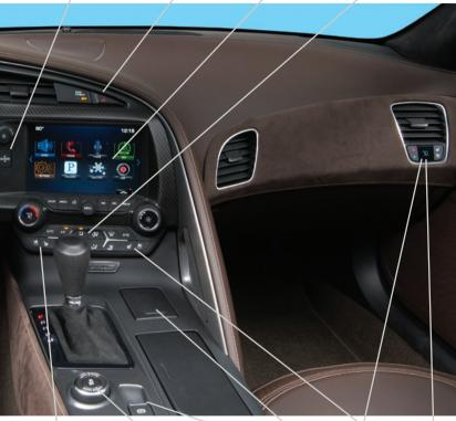
Driver's Heated/ Ventilated Seat Control\* Driver Mode Control/Stability Control Button Electric Parking Brake Switch
