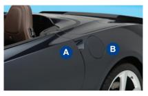
Fuel Door: The vehicle must be unlocked to open the fuel door. With Passive Locking active, the driver's door must be opened first before the fuel door will unlock. Press and release the center rear edge of the fuel door (B) to open it.
