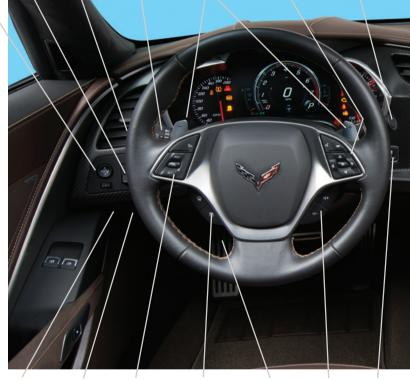
Trunk/Hatch Release Button Advanced Theft Protection Button Cruise Control Buttons Audio Next/ Previous Favorite Station Controls Tilt/Telescopic Steering Wheel Control Audio Volume Controls Engine Start/Stop Button
