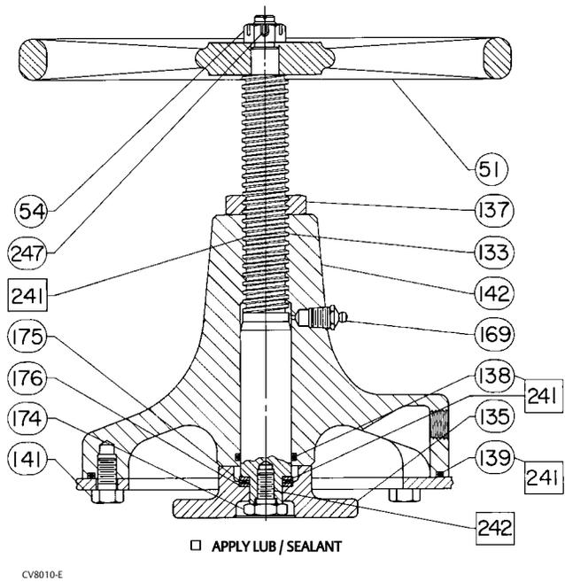
TOP-MOUNTED HANDWHEEL ASSEMBLY FOR SIZE 70 ACTUATORS
