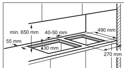
If several 30 cm hobs are to be installed side by side into the same cut out, an assembly kit including a support side bracket and supplementary seals is available at our Service Centres. The relevant installation instructions are supplied within the kit package.
