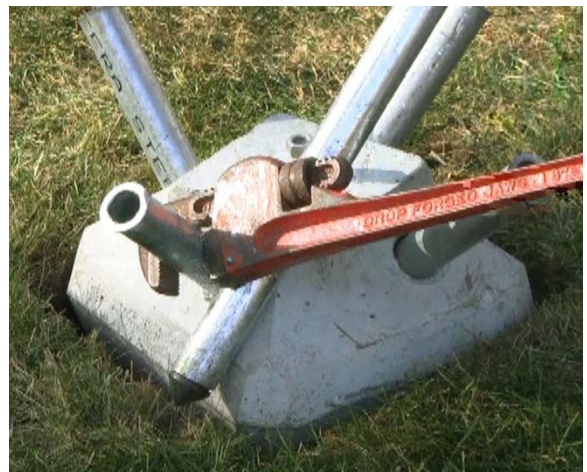
Figure 6. Jacking Method for Pin Removal
