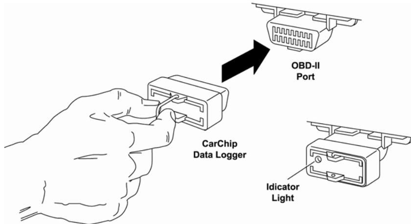
3. Check to make sure the data logger indicator light is blinking. This verifies CarChip was properly inserted into the OBDII port and is communicating with your vehicle.
