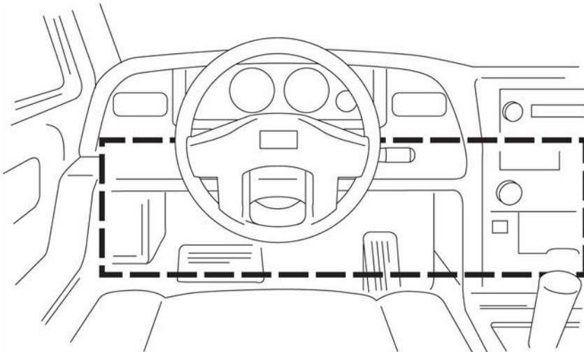
**Note:** If you have trouble finding your OBDII connector, don't forget to look under the dash or in the dash area in front of the passenger seat.
