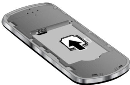
3. To remove the SIM, slide it gently out of the socket.
