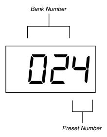
To change presets within a bank, simply step on one of the buttons numbered 1 through 5. The last digit in the display will change, and the MasterMind will send the MIDI commands associated with the new preset.
