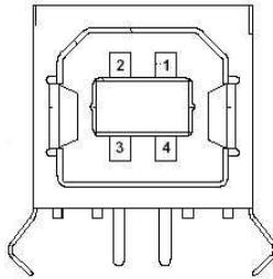
Fig. 6.3-2 USB “B” type connector
