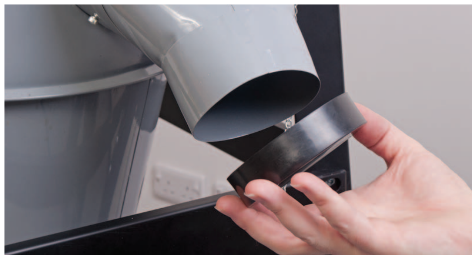
Inlet manifold with removable lid
