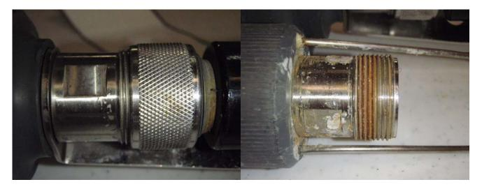
(Above Left) Example of a correctly mated connector. Note: There are typically only two exposed threads when the connector is fully inserted and o-rings are sealed.
