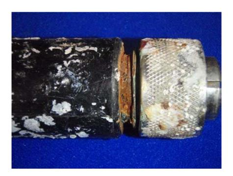
(Above) Example of a cable connector that did not have the locking sleeve fully engaged with the sonde connector. Water infiltrated the sonde connector and caused a short that corroded the cable connection from the inside.
