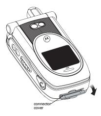
With the Smartphone's display facing up, insert the serial data cable's connector into the accessory connector, until you hear a click.
