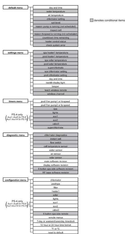
The Default Menu is a series of informative displays (temperatures, salt levels, chlorinator settings, etc.) with nothing to set. The Aqua Logic will automatically switch to the default menu when no keys have been pressed for 2 minutes and will then scroll through each display.
