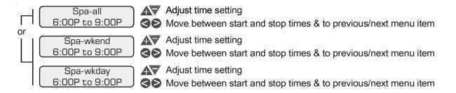
This menu is only available if the system has been setup for "spa only" or "pool and spa". During the programmed spa time, the Aqua Logic will turn on the filter pump and move the pool/spa valves into the "spa-only" position. The heater will automatically heat the spa up to the programmed spa temperature (page 7). This programmed spa operation will take precedence over all other automatic functions, only manual operation of the filter button or pool/spa valve button will override this function.
