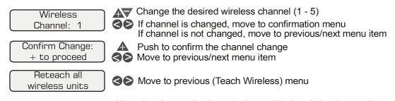
This setting changes the channel to be used by the wireless base station and remote(s). If the channel is changed and confirmed, all of the wireless remotes will have to be retaught. This menu will only appear if a wireless base station is connected to the Aqua Logic.
