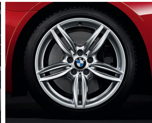
19" M light alloy wheels Double-spoke 351 M with mixed tyres , front 8.5 J x 19 with 245/40 R 19 tyres, rear 9 J x 19 with 275/35 R 19 tyres.
