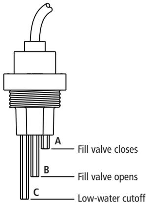
Systems using tap or softened water control water levels electronically using a three-rod probe. The controller responds with the above actions when the water level reaches each rod.
