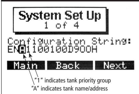
Humidifier tanks ordered as a multi-tank group are configured at the factory. The configuration process includes:
