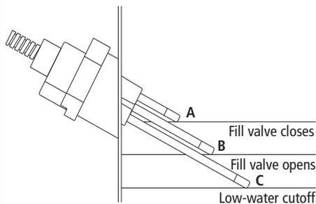
Systems using tap or softened water control water levels electronically using a three-rod probe. The controller responds with the above actions when the water level reaches each rod.
