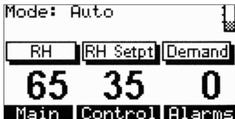
This is the Idle Screen displayed with Vapor-logics versions 2.x.x, 3.x.x, 4.x.x and 6.x.x
