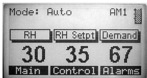
This is the Idle Screen displayed with Vapor-logics versions 5.x.x and 7.x.x (systems with multi-tank configuration capability)
