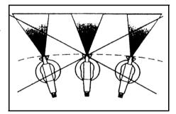
When spraying large areas, using a criss-cross pattern as shown.
