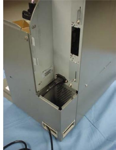
**Figure 2h. Plugging the power cable**
