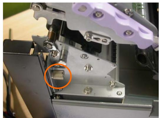
Figure 1b. Removing the thumbscrew that secures the front cover.
