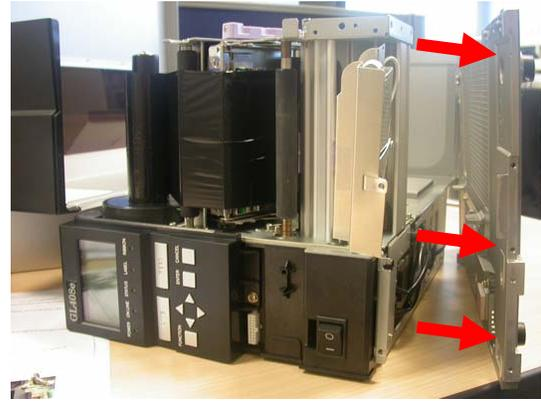
**Figure 1h. Separating the base from the printer**
