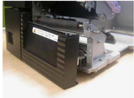
Figure 1c. Front cover can now be removed
