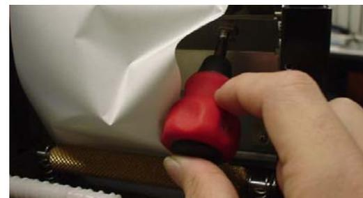
**Figure 3c. Adjusting liner meandering via the adjust collar.**
