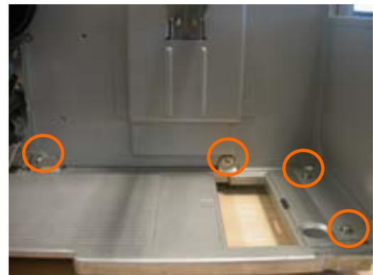
Figure 1d. Removing the lock shaft.
