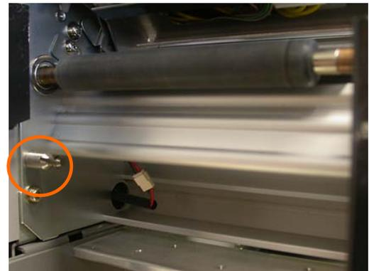
Figure 1d. Removing the lock shaft.
