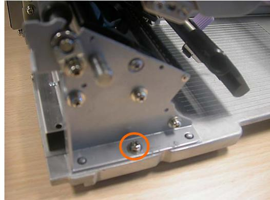
**Figure 1e. Removing the fifth of nine screws**
