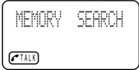
2. Press **RING/VOL** or **ON/OFF MUTE** as needed to locate the number in Memory.
