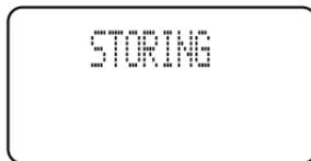
**Note:** *In storing a number operation, you must press a key within 20 seconds. Otherwise, an error tone sounds and the unit returns to standby mode.*
