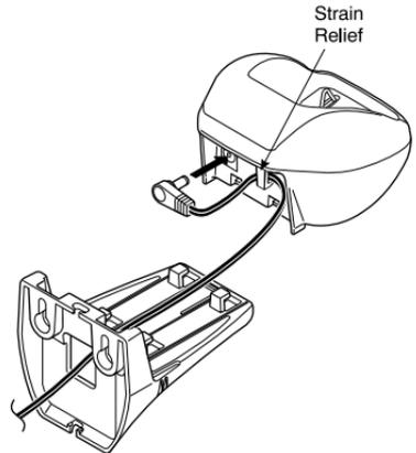
3. Slide the wall mount stand into the notches on the bottom of the charging unit.
