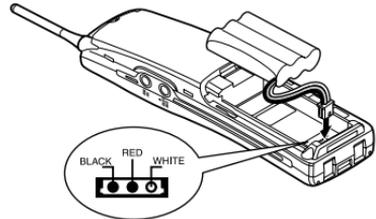
3. Place the cover and slide the cover up until it latches into the Handset.
