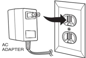
**Note:** Do not use an outlet controlled by a wall switch.
