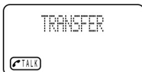
The dialed numbers saved in xfer memory is shown on the display after 2 seconds.
