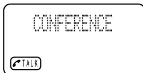
The dialed numbers saved in conf memory is shown on the display after 2 seconds.
