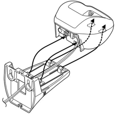
4. Place the Charging Unit on the posts of the wall screws and push down until it's firmly seated.
