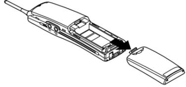
2. Connect the battery pack connector observing correct polarity to the jack inside the battery compartment.
