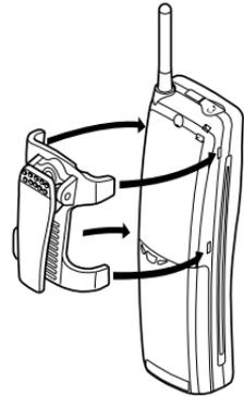
2. Slide the clip into the tab slot.
