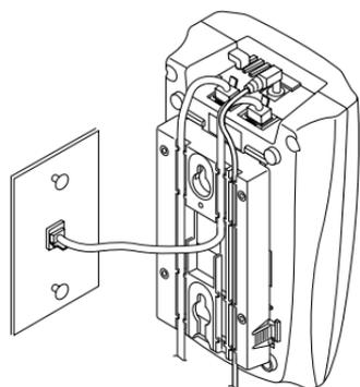
4. Plug one end of the telephone cord into the **LINE** jack on the Base Unit. Optionally, plug one end of a standard 2500 type desk phone into the **PHONE** jack. Then place the telephone cord(s) inside the molded channel(s) on the bottom of the Wall Mount stand.
