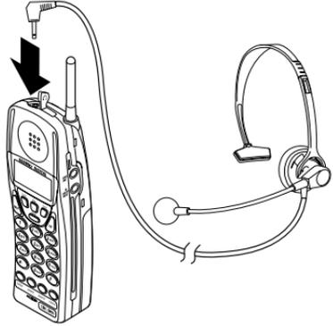
Operation of the **ANA 9310** using the Headset is exactly the same as that of without Headset. Only the difference is, you will hear through the Headset earphone, and talk through the Headset microphone. The Handset earphone and microphone (mouthpiece) are disconnected.
