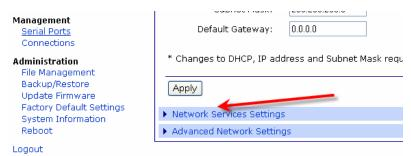
The only Network Services that should be enabled are TCP sockets are ADDP and HTTP.
