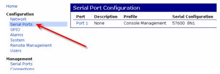
8. Click on Port1, to display its configuration. The Port Profile should be "TCP Sockets" as shown below. If it does, skip to step 5, if not, perform step 4.
