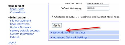
7. In Network Service Settings, highlight only the service you wish to use. For Telenet, the minimum recommended is: ADDP, Telnet, and HTTP.
