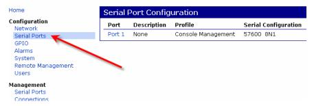
3. Click on Port1, to display its configuration. The port profile shoul dbe "Console Management" as shown below. If it does, skip to step 5, if not, perform step 4.
