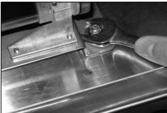
Removing the assembly mounting nuts.
