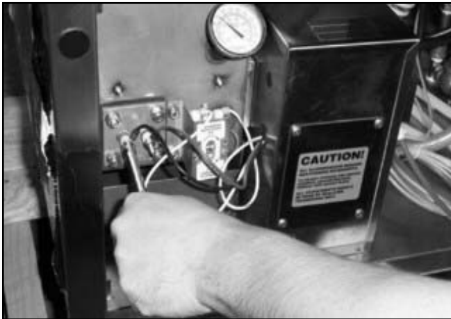
Removing the heater nuts.
