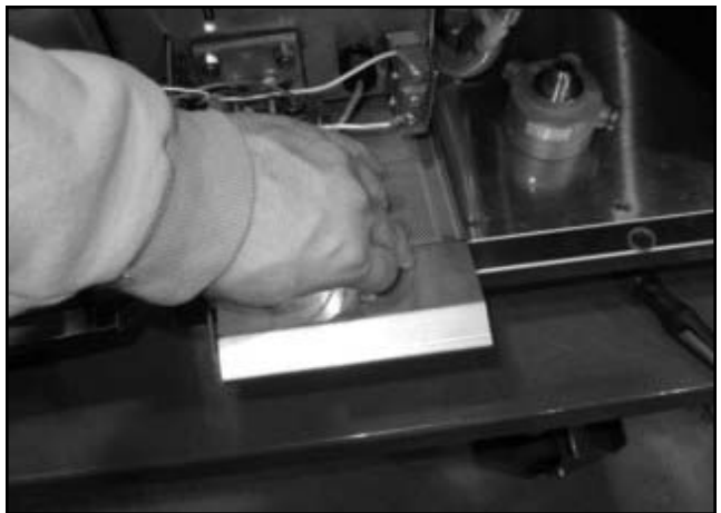
Removing the lower strainer.
