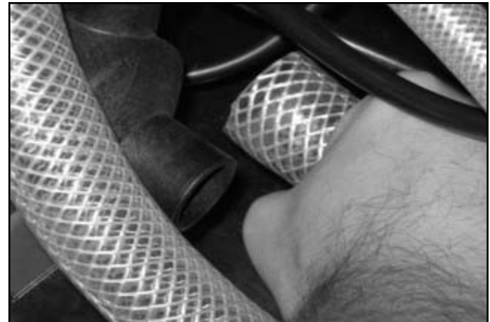
Suction hose coming off when moving the assembly.
