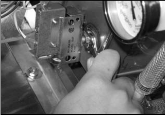
Removing the probe and imperial brass fitting.
