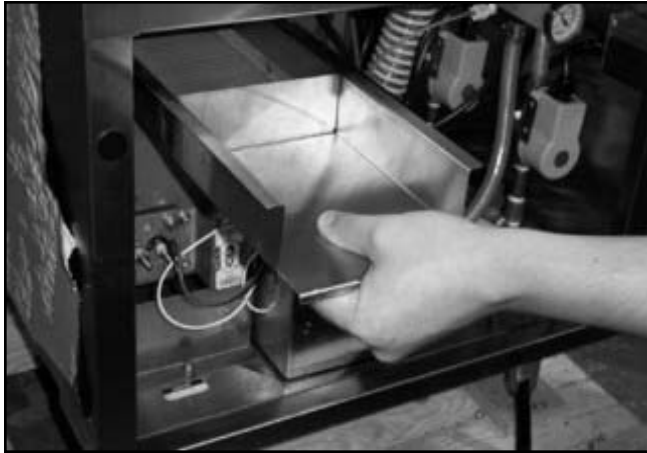
Removing upper (wash) strainer.
