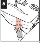
Rebuckle belt. Lap belt portion should now be tight. If not, remove locking clip and repeat all steps.
