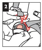
Push each buckle plate into buckle until you hear a "click". Remember to always pull up on harness straps to make sure buckle is locked tightly.
