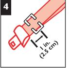
Position locking clip about 1 in. (2.5 cm) from vehicle belt's buckle plate.
