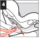
Thread the vehicle lap belt or lap/shoulder belt combination through the belt path and out other side. Buckle.
