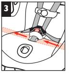
Thread UNDER seat pad behind the crotch strap, between crotch strap and rear harness slot, and out opposite side. Buckle vehicle belt.
