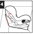
Place child restraint rear-facing in the back seat. With child restraint in the fully reclined position, make sure level line on side of shell is level with ground. Adjust
