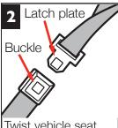
Twist vehicle seat belt and latch plate (or buckle)
