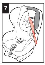
From the front, pull pad off the shell, starting at the top. Lift pad over the harness strap holders and work the pad around the harness adjustment cover.
