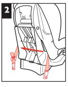
Adjuster MUST be on the left side of child restraint as shown. DO NOT twist belt.
