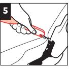
Fasten one LATCH belt connector to the anchor in the vehicle seat located in the vehicle seat bight. Repeat for other side of child restraint. See your vehicle owner's manual for more information.
