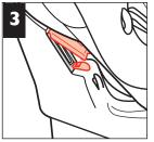
Open the lock-off opposite of the vehicle buckle by press down on the lock-off's tab.
