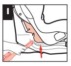
Recline child restraint. To thread the LATCH belt, put belt end with connector and adjuster through the forward -facing belt path slot.
