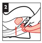
Thread the vehicle lap or lap/shoulder belt combination through the rearfacing belt slot.
