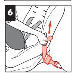
Place one knee in the child restraint and push down firmly while pulling up on loop end of the LATCH belt to tighten.
