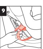
Pull out the harness and splitter plate.
