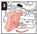
Rotate the recline foot to the front of the restraint and lock into place.
