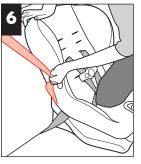
Place one knee in the child restraint and push down firmly while pulling up on shoulder belt to tighten. For a manual belt, refer to "Knowing your Vehicle Belt" section.
