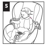
Place the child's bottom and back flat against the child restraint. This will increase comfort and allow the harness to properly tighten.
