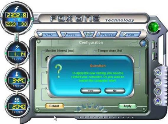
Later on, when the FOX ONE program is activated, and F.I.S. feature (in CPU Page) is also enabled, FOX ONE will automatically adjust your CPU clock according to your system loadings. (Loadings are like Power Gaming, Data Mining...etc.)
