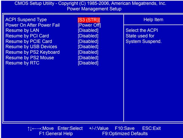
ACPI (Advanced Configuration and Power Interface) is an open industry standard interfaces enabling OS-directed configuration, power management, and thermal management of mobile, desktop, and server platforms. It defines five sleeping states, they are :
