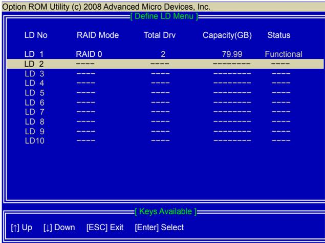
9. You can see in the previous example, about 40GB of Channel 1 and 2 hard disks were allocated. Select the remaining spaces from them for RAID0 again. Press [Ctrl-Y] to save the setting.
