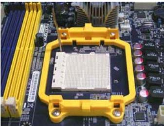
1. Release the CPU socket lever.
