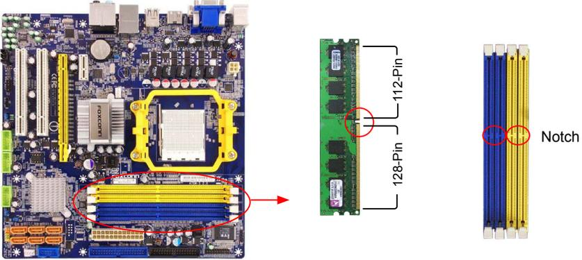
If you take a look at front side of memory module, it has asymmetric pin counts on both sides separated by a notch in the middle, so it can only fit in one direction. Follow the steps below to correctly install your memory modules into the sockets.
