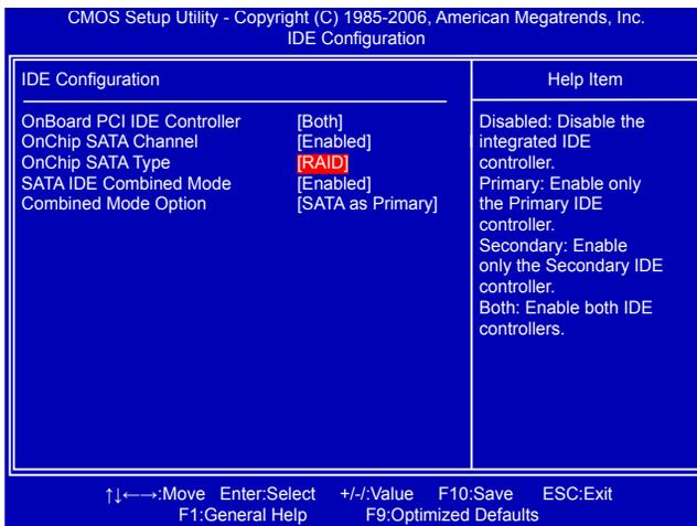
2. Select a RAID array for use (also can refer to section 5-3)
