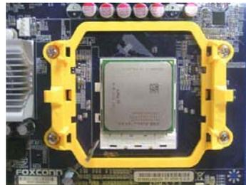
2. Align pin one of the CPU with the CPU socket, and gently put the CPU onto the socket.
