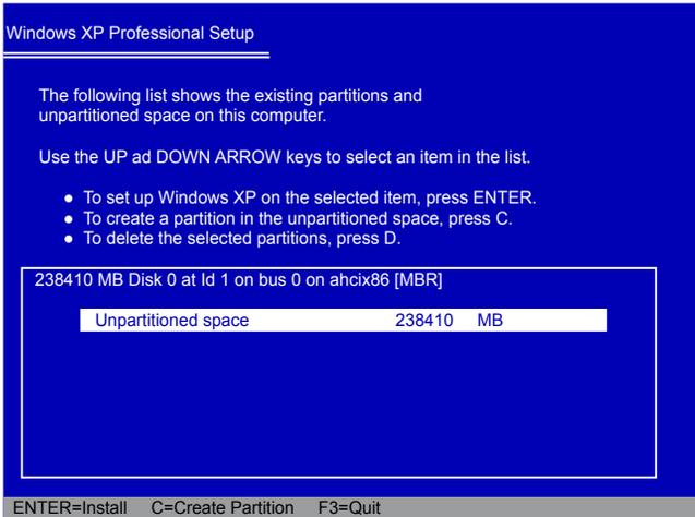
10. In this example, we will create a 30GB partition C: and leave the remaining space as a partition E: (D: is allocated by a DVD drive)
