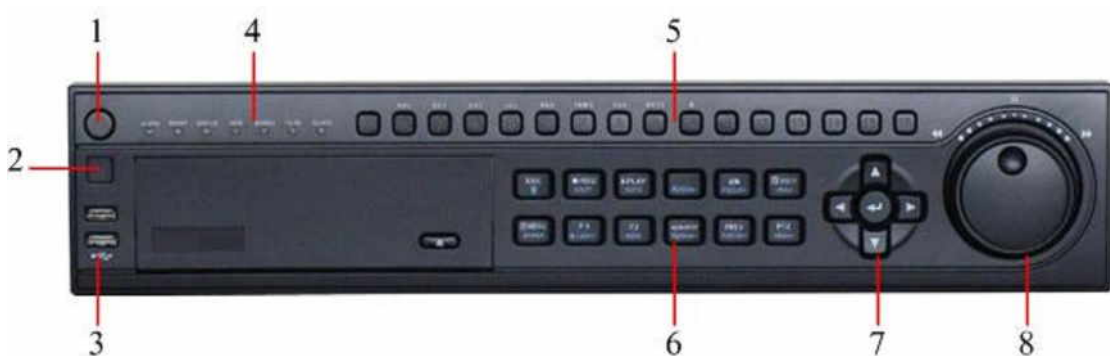
Figure 3. DVR Front Panel Controls
