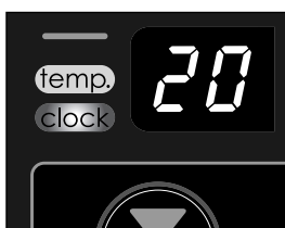
F: When the CLOCK indicator light stops blinking, the setting has been locked to the indicated value.
