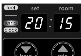
G: The required temperature on the left, the measured temperature on the right.
