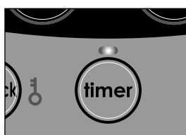
H: The TIMER indicator light indicates that the timer function has been switched on.
