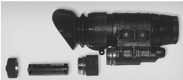
Figure 4-2 DNAAS Battery Installation.
