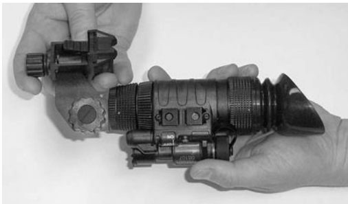
Figure 3-3 Attaching ATN NVM-14 to Headmount Adapter
