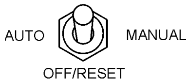
Figure 55. MPEC Control Switch (Off/Reset)
